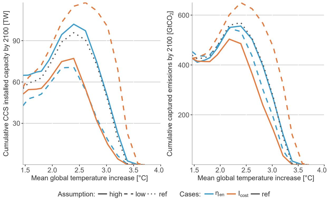
Figure 4: Variation in installed CCS capacity and CO<sub>2</sub> captured emissions over temperature increase, in response to changes in efficiencies and investment cost
